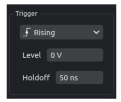
The trigger level ranges from –950 to +950 mV, and can be set with 12-bit resolution. The trigger level may also be changed by dragging the yellow **T** marker on the right side of the main display.
