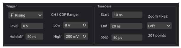
In this mode, the timebase start, stop, and step can be set manually. The timebase can be extended up to the smallest post-trigger delay allowed by the hardware; this is unit-dependent, but is generally 8 ns or earlier. Channel 1 will experience increased distortion in this region.
