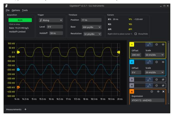
Reference any of the available channels using **CH1**, ..., **CH8**. The math feature can be combined with the de-embedding tool.
